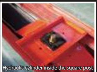
Hydraulic cylinder inside the square post
